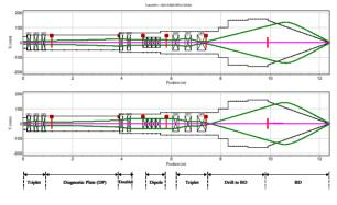
Figure 2: 3 RMS envelope for HEBT line.
