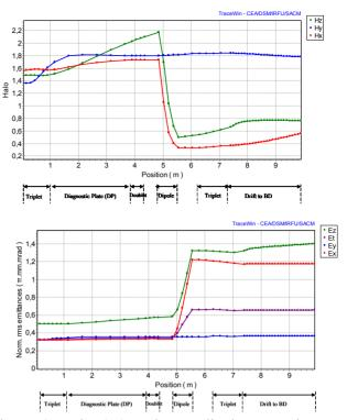
Figure 4: Halo (up) and normalized rms emittance (bottom) in the HEBT. X and y are the transverse coordinates whereas z is the longitudinal one.
