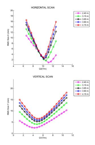
Figure 1: Quadrupole scan for transverse emittance measurement. RMS beam size as a function of the quadrupole gradients (first quadrupole for the horizontal direction and third for the vertical one). The different curves show the rms sizes at different locations from the input of the HEBT.
