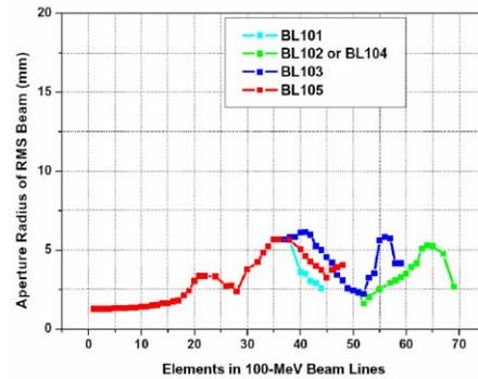
Figure 7: rms beam size in each element of PEFP 100 MeV beam lines.
