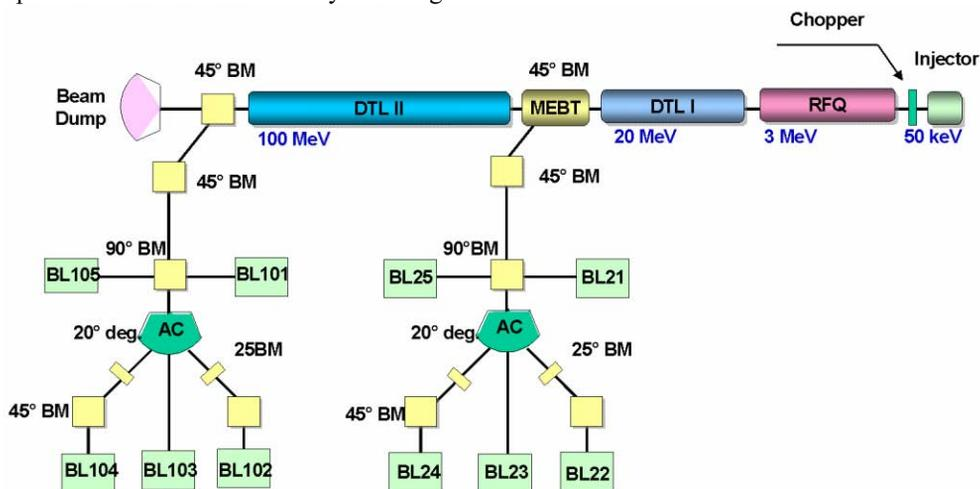
Figure 1: Schematic plot of the PEFP linac and beam lines. 20 MeV proton beams are extracted by a 45-degree bending magnet located in the MEBT and 100 MeV beam lines begin from a 45-degree bending magnet after the linac. The bending angles are explicitly given for the dipole magnets.
