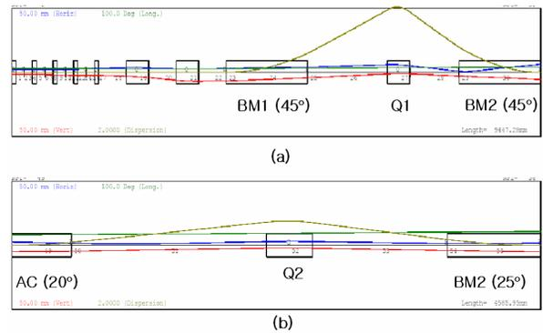
Figure3: Dispersion free condition in 100-MeV beam lines: (a) between two 45-degree bending magnet and (b) between AC and 25-degree dipole magnets. The boundary of figure represents the dispersion value of 2 m.
