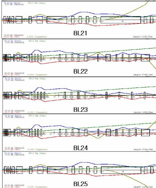
Figure 4: Beam optics results of PEFP 20-MeV beam lines.
