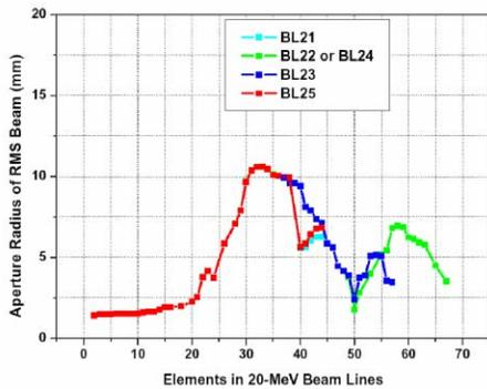
Figure 5: rms beam size in each element of PEFP 20-MeV beam lines.
