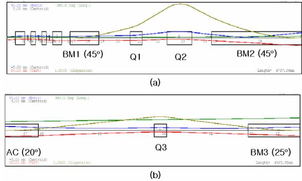
Figure 2: Dispersion free condition in 20-MeV beam lines: (a) between two 45-degree bending magnet and (b) between AC and 25-degree dipole magnets. The boundary of figure represents the dispersion value of 1.5 m.
