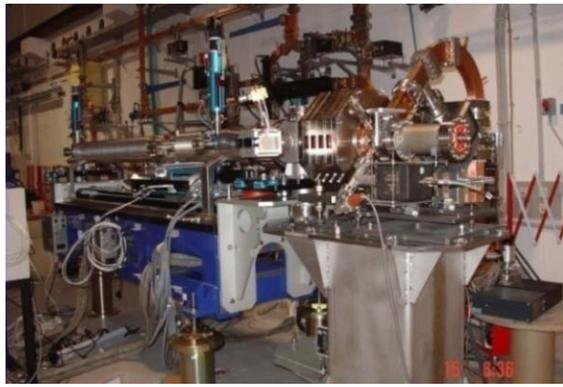
Figure 5: The RF Gun and the emittance meter (long bellow on the left) at SPARC.
