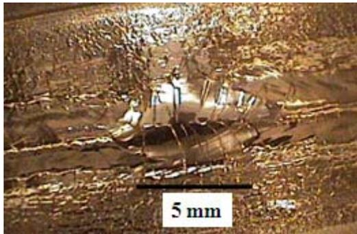
Figure 8: Starting or ending point of electron beam welding.
