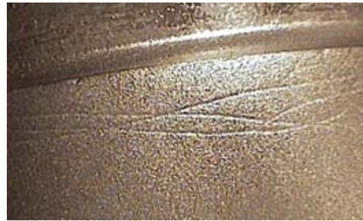
Figure 10: Scratches near the equator.
