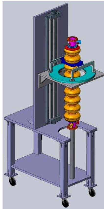
Figure 2: Cavity inspection hardware with a 1.3 GHz 9-cell cavity. The videoscope and the motors for moving the cavity are not shown here.
