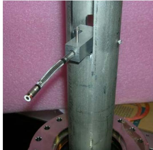
Figure 5: A 6 mm diameter videoscope set in the fixture.
