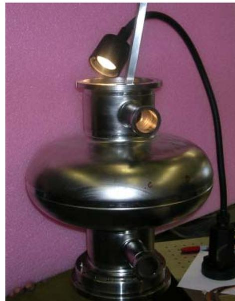
Figure 6: A 805 MHz single-cell cavity inspected.
