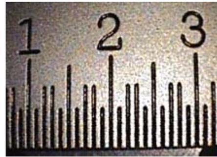
Figure 4: An image of a scale using a 5 mm videoscope. The smallest increment between lines is 254 microns.
