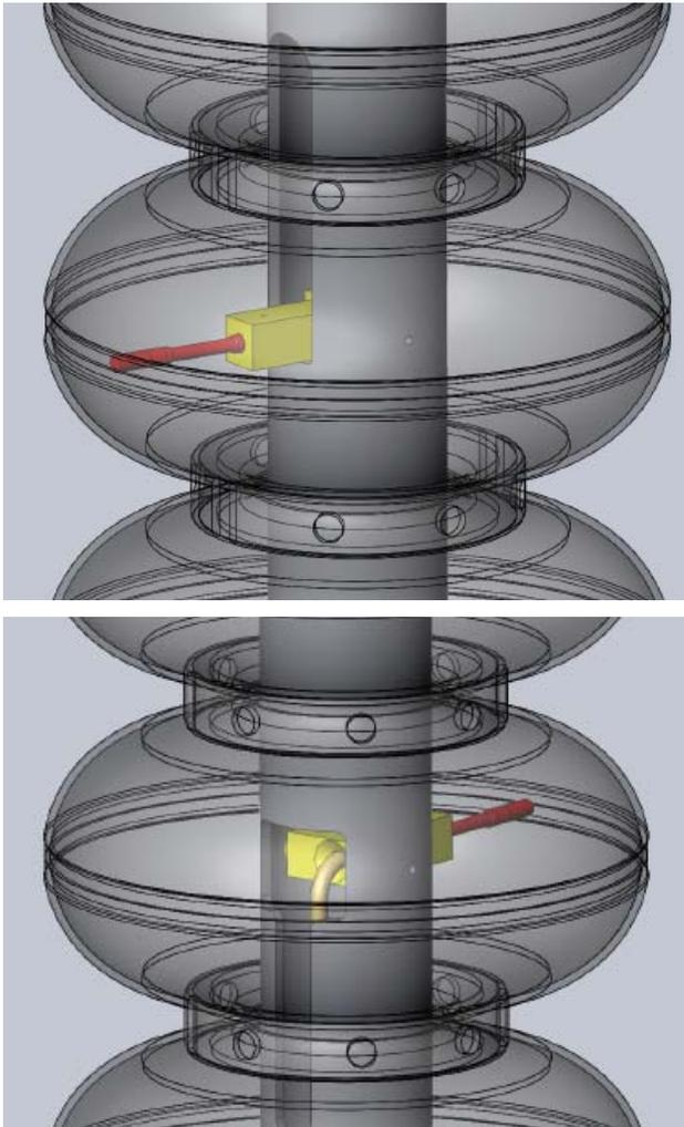
Figure 3: Schematic of a 6 mm videoscope inserted in the cavity. The closest distance to the cavity will be 4-7 mm depending on the scope you choose.
