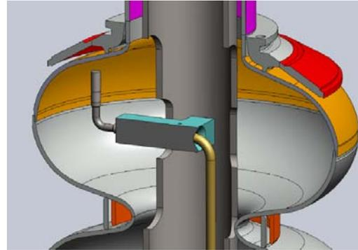
Figure 1: Conceptual drawing of the surface inspection using a videoscope.
