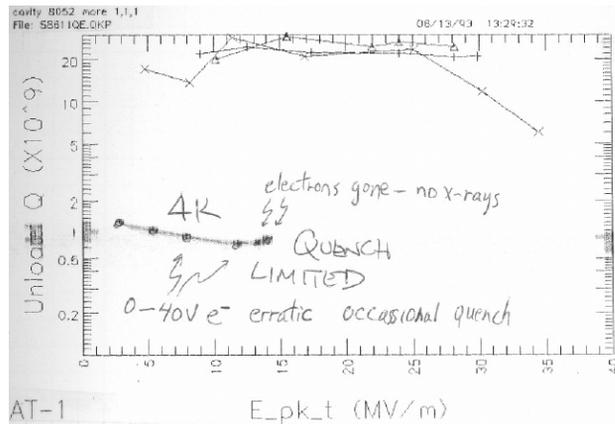
Figure 7: 805MHz single-cell cavity  $Q_0$ - $E_{\text{peak}}$  curve measured on 13 August 1993.
