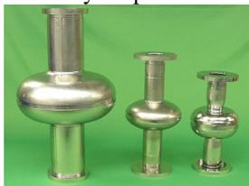
Figure 2: Single crystal cavities (left: TESLA-type, 1.3 GHz, center: HG, 2.3 GHz, right: ILC\_LL, 2.3 GHz).
