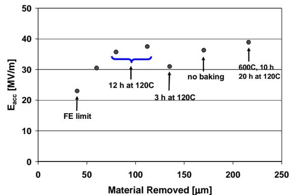
Figure 3: Evaluation of gradient with material removal.
