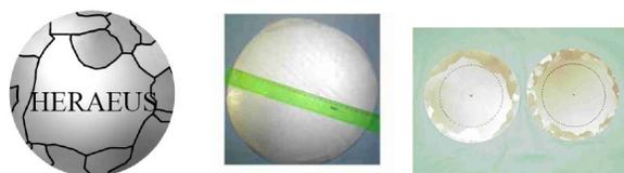
Figure 1: W.C.Heraeus (left: large grain, center: enlarged grain) and CBMM (right) material used for the fabrication of single crystal cavities.
