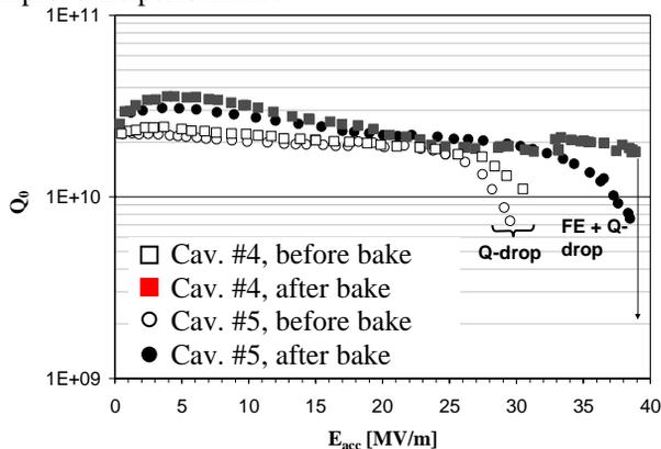
Figure 4:  $Q_0$  vs.  $E_{acc}$  at 2 K for single crystal cavities #4 and #5 (best performance).
