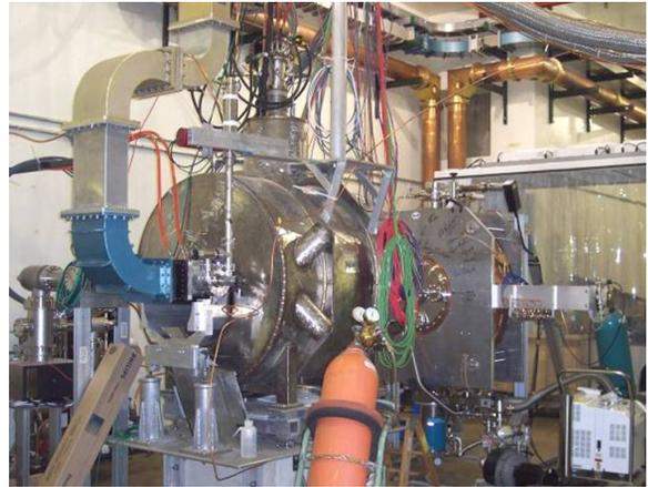
Figure 8: The 201-MHz prototype cavity was installed and tested at MTA, FNAL since 2005.
