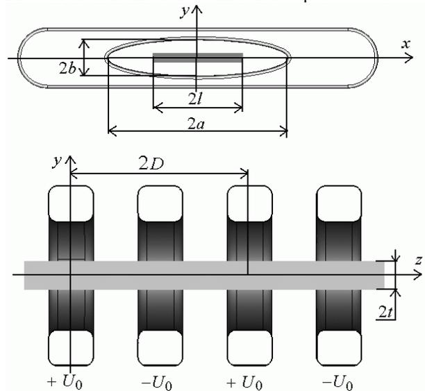
Figure 3: The general view of electrostatic undulator.
