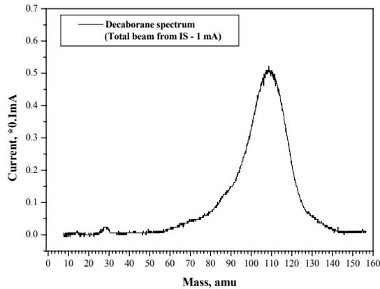
Figure 1: Mass spectrum from ITEP Bernas ion source.
