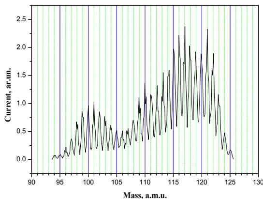
Figure 2: The decaborane beam spectrum with high resolution.
