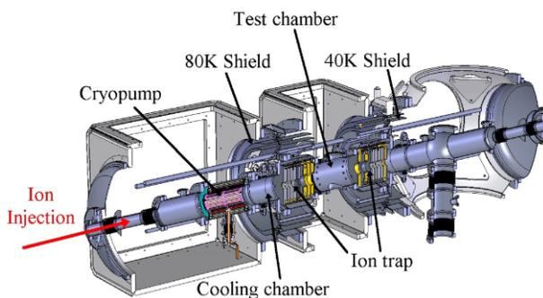
Figure 3: Scheme of the prototype with ion trap, cooling units, cryopump and cooling tubes.
