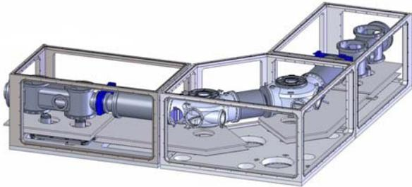
Figure 4: Design drawing of one corner. The frames of the outer chambers and the inner cold chambers are visible. Large rectangular flanges allow easy access.
