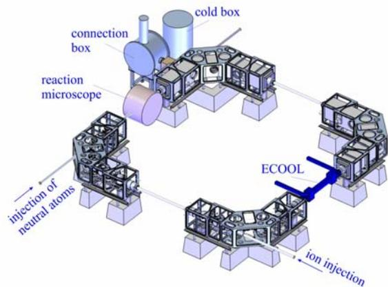
Figure 1: Schematic layout of the CSR with the internal targets and some components of the refrigerator.
