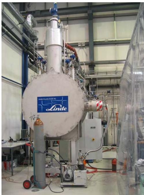
Figure 2: The connection box with a height of about 5 m and a diameter of 1.6 m. At the right side (red stripes) a heater box for acceptance tests is visible. After removing the heaters the connection box was coupled to the experiment.
