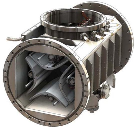
Figure 5: The ion-optic cell with the quadrupole electrodes. On the left the evaporation helium line is visible.
