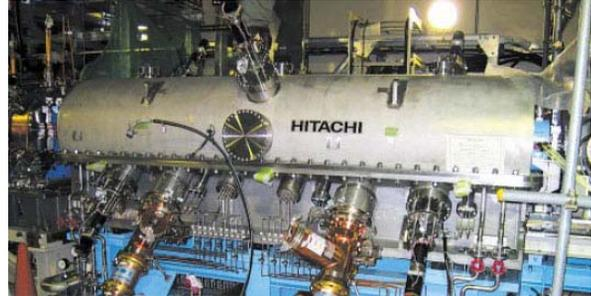
Figure 1: RFQ linac for the first-stage of the accelerator.
