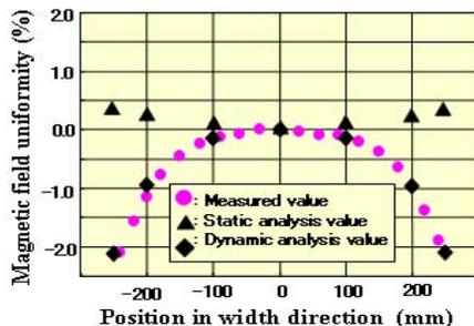
Figure 5: Magnetic field uniformity in the case of a horizontal shift bump magnet.
