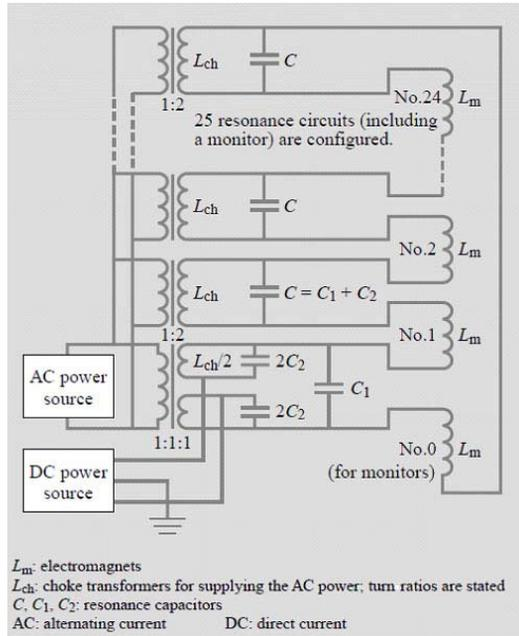
Figure 3: Power supply system for the BMs
