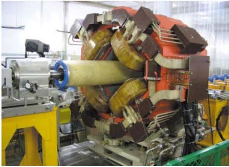
Figure 2: A QM during magnetic field measurements.
