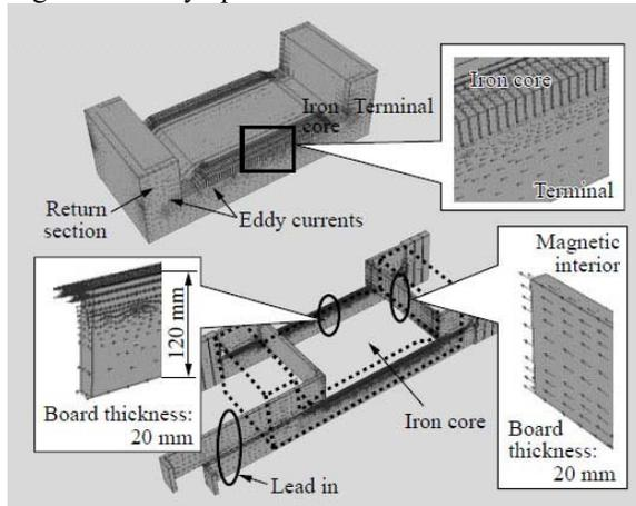
Figure 4: Eddy current distribution obtained from the electromagnetic analyses of a horizontal shift bump magnet.
