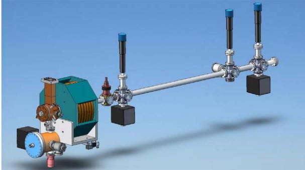
Figure 2: Setup for testing the 2998 MHz photo-cathode rf gun
