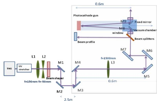
Figure 4: Optics for laser beam transport and virtual cathode.
