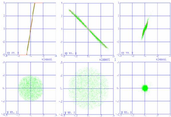
Figure 6: Electron distributions in x-y plane (lower plots) and transverse trace space (upper plots) at gun exit (left), after the emittance compensation solenoid (middle) and at second emittance minimum in the drift section (right) respectively.
