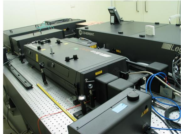
Figure 3: The UV drive laser for the 2998 MHz photo-cathode rf gun.
