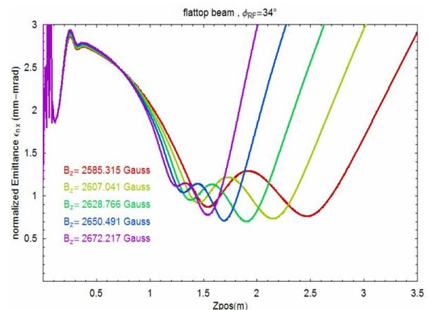
Figure 5: Evolution of normalized emittance at various solenoid magnetic field strength for a 10 picoseconds ideal temporal flattop electron beam.
