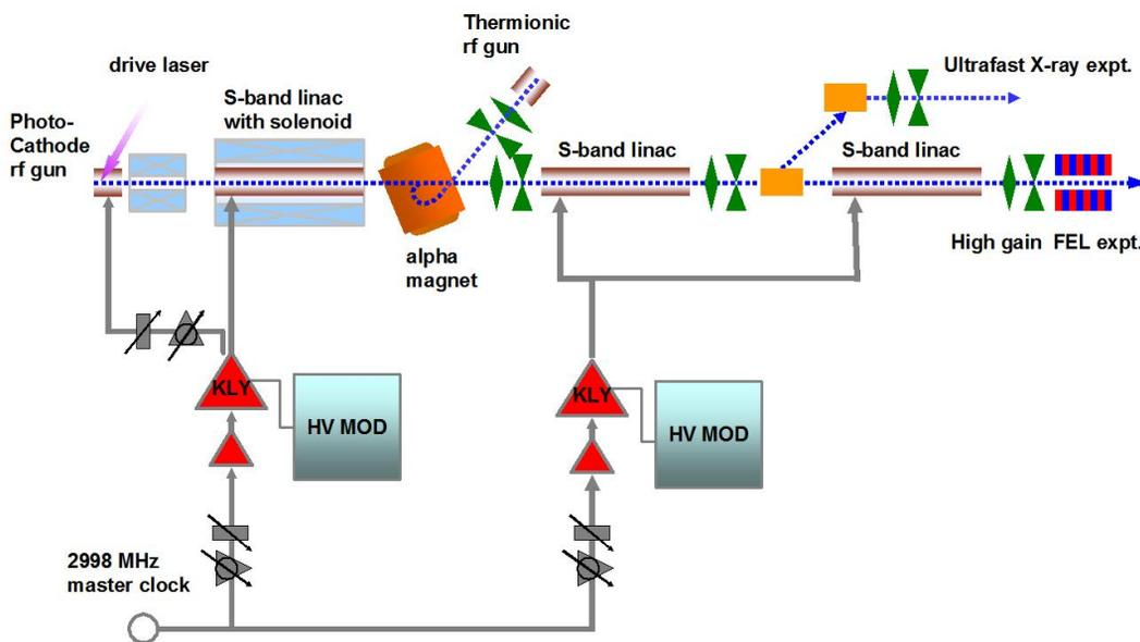
Figure 1: The NSRRC high brightness injector system
