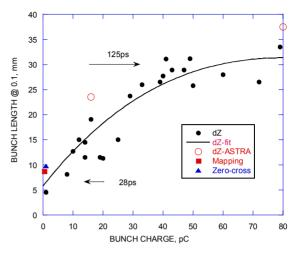
Figure 3: Bunch length at 10% of the peak value as a function of bunch charge. Data were obtained with the RF transverse kicker (full circles), "energy mapping method" (square) and zero-crossing method (triangle). Open circles are the results from the ASTRA model.
