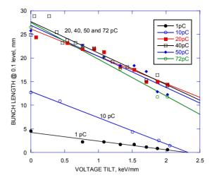
Figure 6: Bunch length at the position of the transverse kicker as a function of the voltage (energy) tilt introduced by the buncher.
