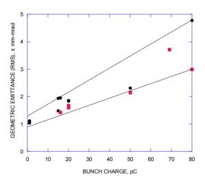
Figure 2: Horizontal (circles) and vertical (squares) RMS geometric emittance as a function of the bunch charge. The straight lines indicate boundaries within which all measured values are contained.
