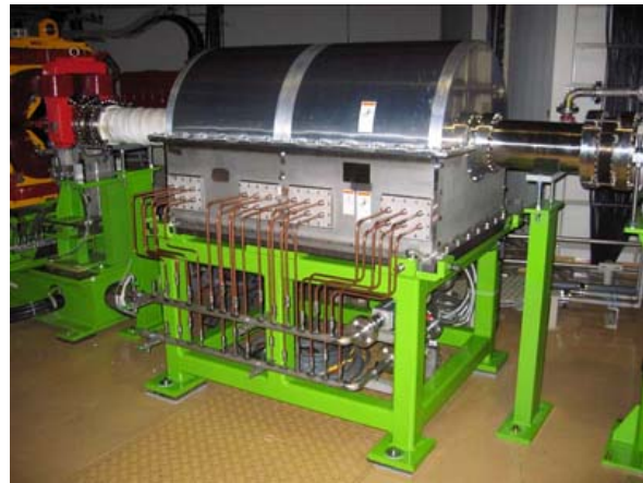
Fig. 3. Acceleration cavity installed in the HIMAC synchrotron for beam test.
