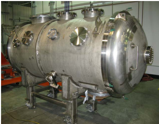
Figure 4: Horizontal Cryostat Assembly
