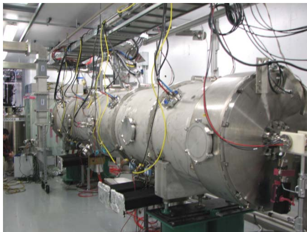
Figure 3: View of Cryomodule Inside Test Cave
