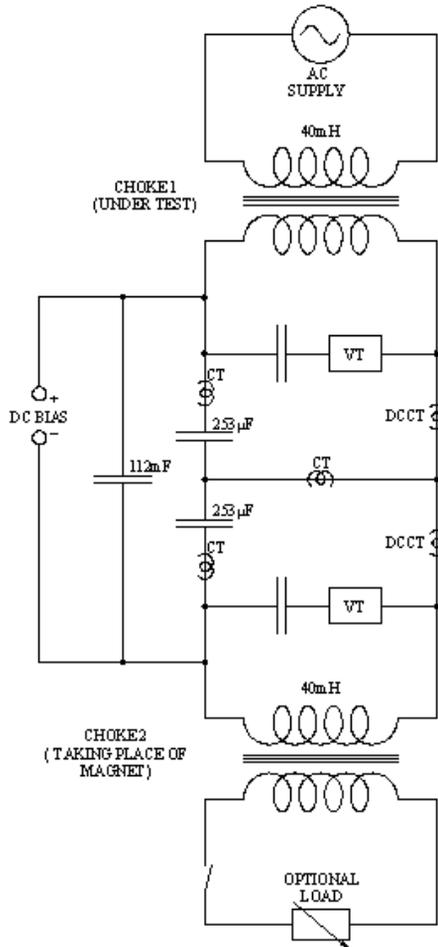
Figure 2: Circuit used for evaluation of model chokes.
