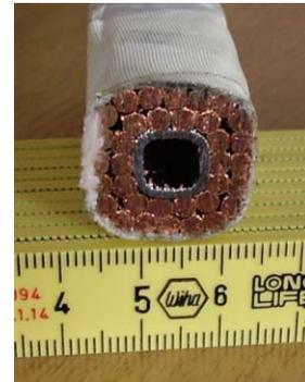
Figure 4: Main winding cross-section.
