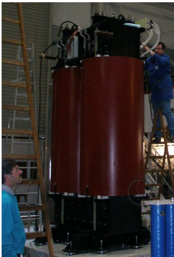
Figure 6: Prototype choke undergoing factory acceptance tests
