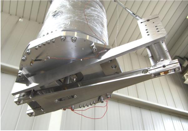
Figure 5: New tuner assembly
