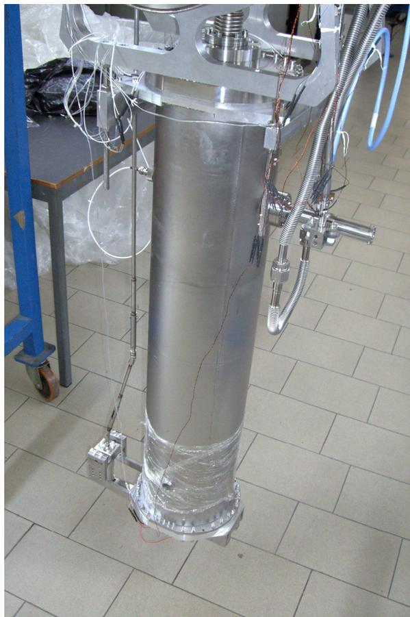
Figure 2: Low- $\beta$  cavity equipped with new tuner and cooled coupler
