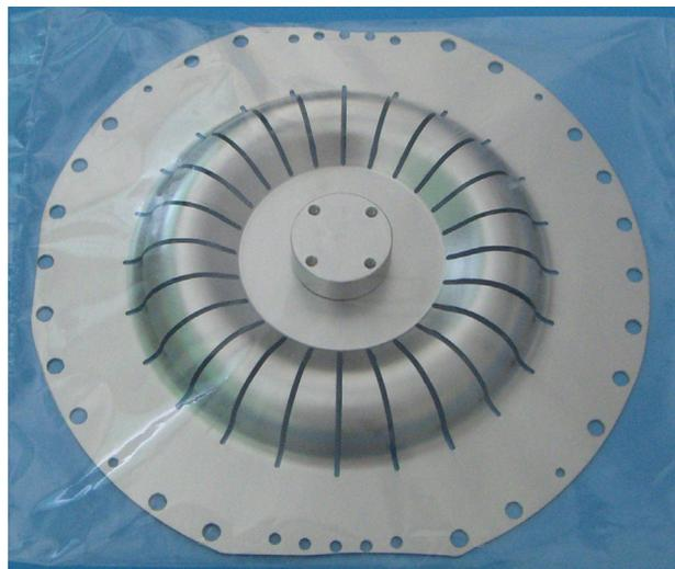
Figure 4: Bulk Nb slotted tuning plate (in a protective plastic bag).
