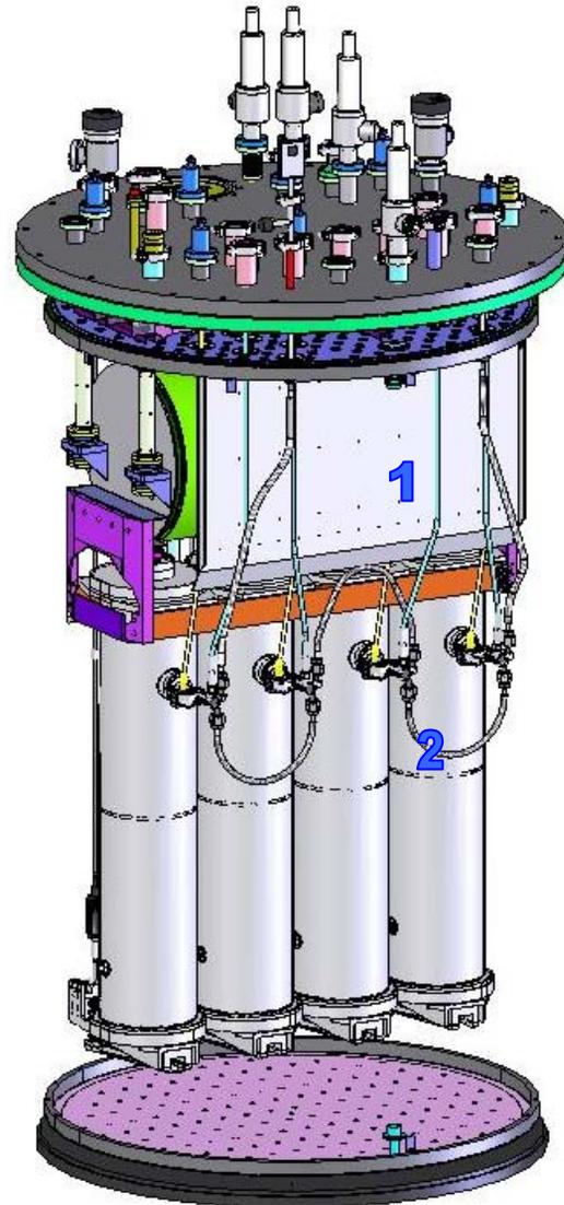
Figure 6: Sketch of the modified cryostat internal part. (1) Aluminum sheet shielding the He reservoir from the rf cables heat irradiation. (2) Flexible cooling pipes bringing LN<sub>2</sub> to couplers.
