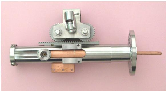
Figure 3: View of the new cooled coupler
