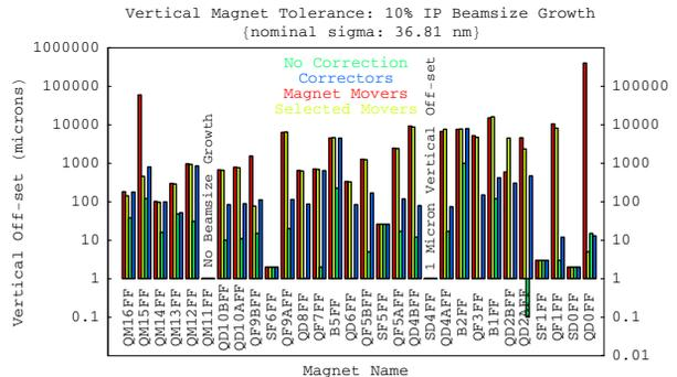
Figure 1: A comparison of the vertical IP beamspace dependency on the vertical misalignment of individual magnets when various orbit correction methods are applied
