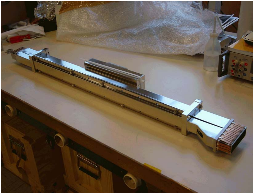
SuperImphy shielding screen around the stored beam chamber
