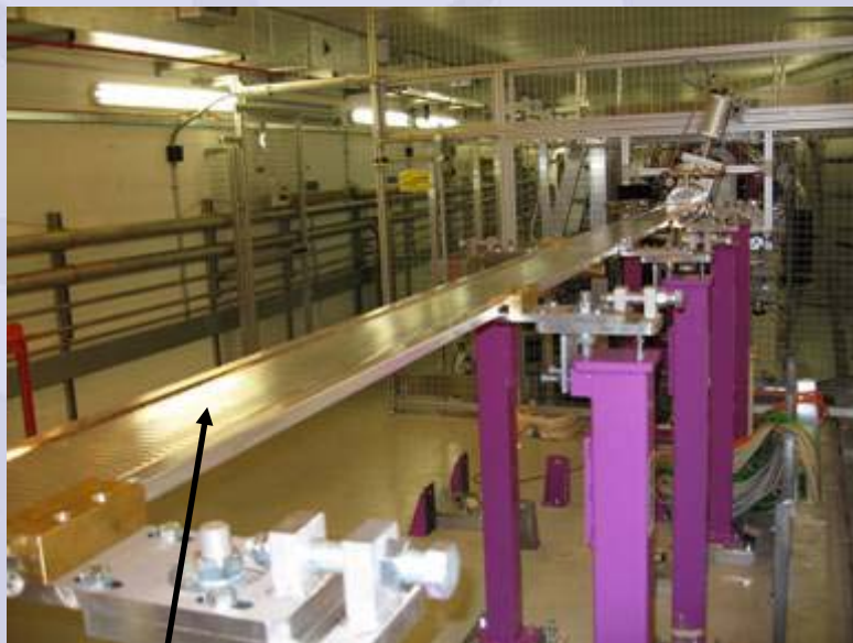
5m long narrow gap vessel for APPLEII undulator
