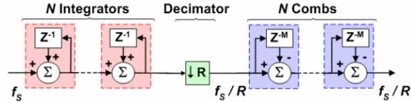
Figure 4: Decimating CIC filter structure.
