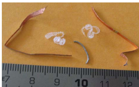
Figure 5: Some of the obstacles found in magnets in the tunnel.
