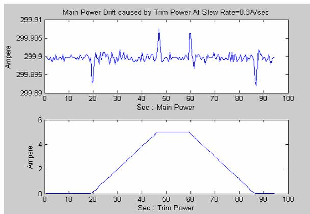
Figure 5: Main power output current@300A SR=0.3 A/SEC vs Trim power current change
