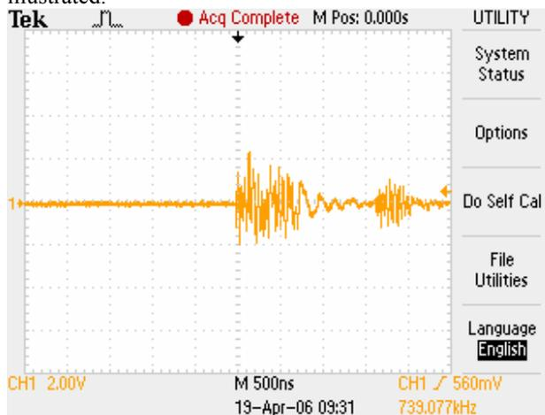
Figure 7: Voltage spike when main power is turned on.
