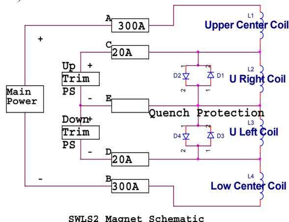
Figure 1: SWLS system connection schematic diagram.
