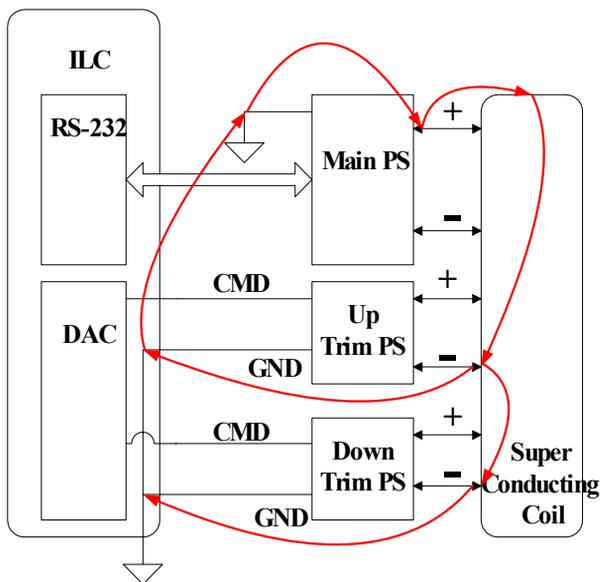
Figure 2: The power supply ground loop in the SWLS system.
