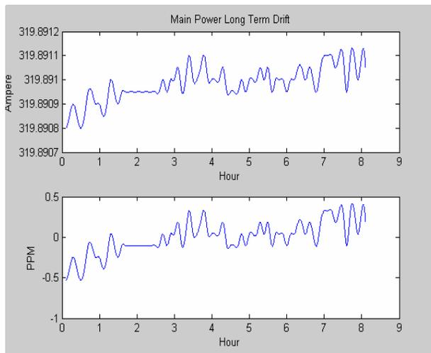
Figure 4: Main power supply long term output current.
