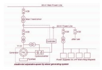
Figure 1: Conceptual block diagram of the power supply system with FWG for 50-GeV MR.
