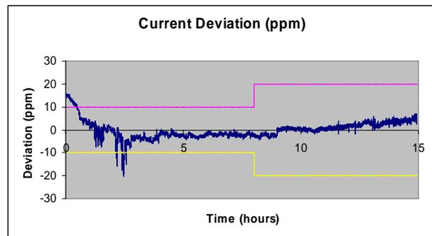
Figure 4: Q Converter Stability
