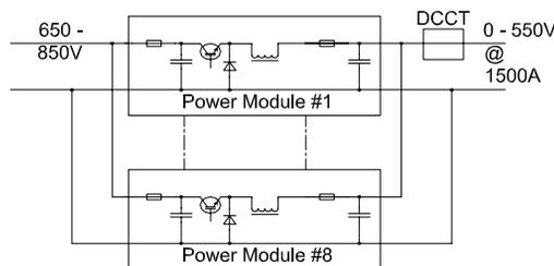
Figure 1: Dipole Converter Topology.
