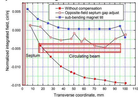
Figure 11: Integrated field distribution before and after compensation
