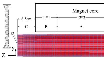
Figure 7: Partitioning of septum conductor
