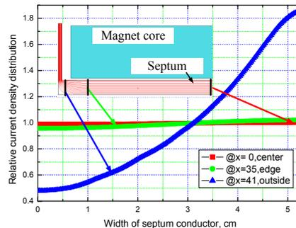
Figure 6: Current distribution in septum conductor
