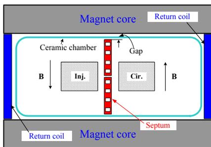
Figure 3: Cross section of opposite-field septum
