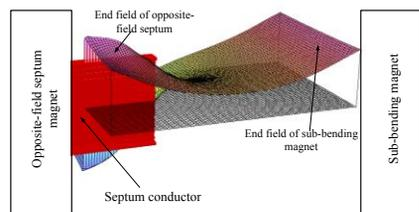
Figure 5: End-field of opposite-field septum magnet
