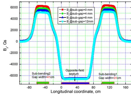
Figure 9: Longitudinal  $B_y$  distribution with different sub-bending magnet gap
