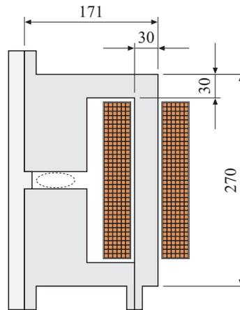
Figure 6: Horizontal Steerer Cross Section
