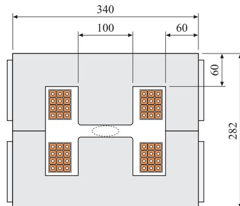
Figure 1: Dipole Cross Section
