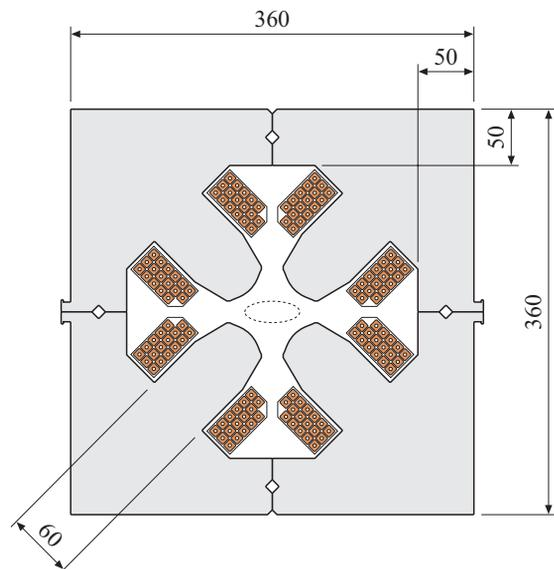
Figure 4: Quadrupole Cross Section
