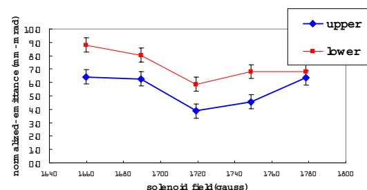
Figure 7: Dependence of normalized-emittance on the solenoid field.
