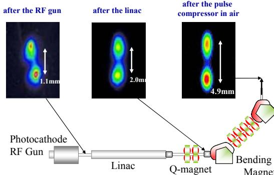
Figure 4: Beam profiles at the exits of the RF gun, the linac and the pulse compressor.
