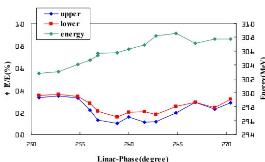
Figure 5: Energy and energy spread versus on the linac RF phase.
