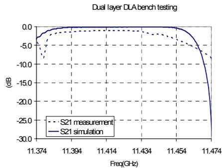
Figure 2: Comparison of the results of the bench testing and the rf transmission simulation of the structure with a single section of double layer ceramic tube.
