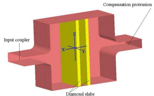
Figure 1: Sketch of cavity design (half shown). Seen are two diamond slabs surrounding the beam channel, the input coupler, and the opposing compensation protrusion to symmetrize the fields. Parameters for the example discussed in this paper are given in Table 1.
