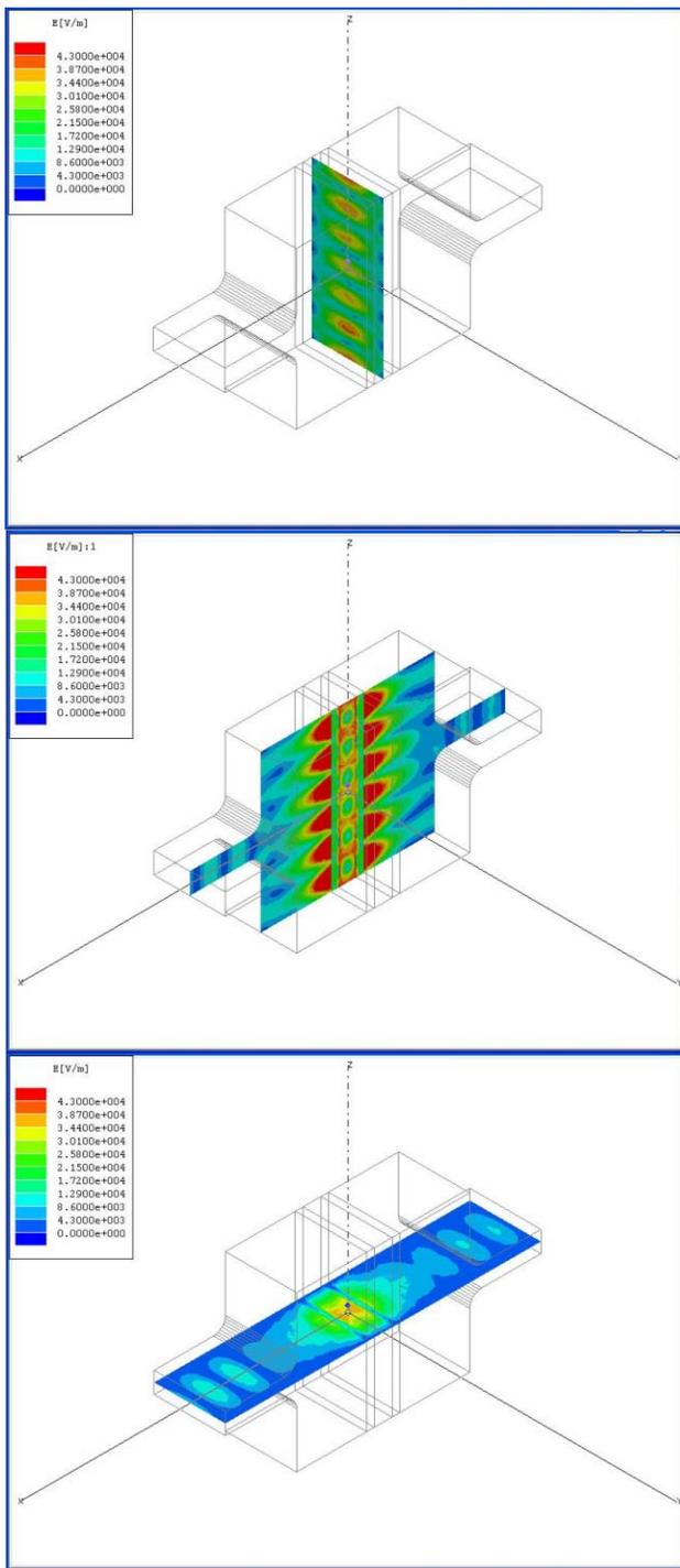
Figure 3: Field pattern in each of the symmetry planes of the operating LSM<sub>216</sub> mode with an input coupler and a compensating protrusion.
