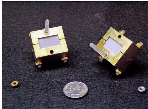
Figure 4: Photo of two halves of LSM<sub>215</sub> mode test cavity that used alumina slabs in place of diamond.
