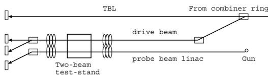
Figure 1: Beam line layout in the CLEX hall.
