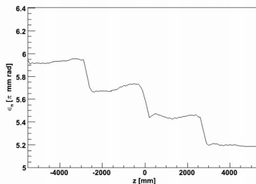
Figure 6: The simulated emittance reduction through the full cooling channel.
