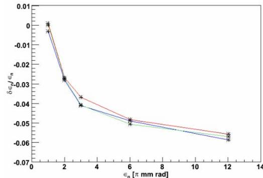
Figure 3: The simulated emittance reduction due to a single liquid Hydrogen block for an absorber with torispherical ends (green), flat ends (blue) and flat ends simulated in ICOOL (red).
