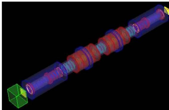
Figure 1: G4MICE visualisation of the central MICE detectors and the cooling apparatus. Time of flight counters are shown in yellow, tracking detector components in dark red, magnet bodies in blue, absorber windows in turquoise and the electron muon calorimeter in green. The distance between the time of flight counters is 13.2 metres.
