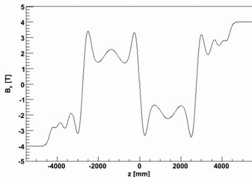
Figure 4: The on axis B-field in the z direction for the MICE baseline case.
