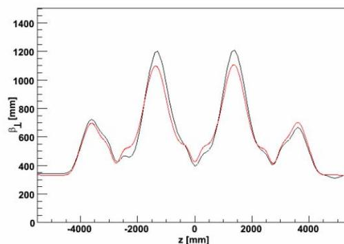
Figure 5: The beta function through the MICE cooling channel from G4MICE's linear optics package (red) and from particle tracking (black).
