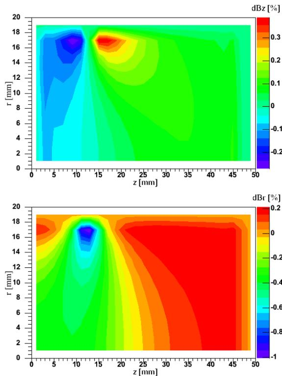
Figure 2: The percentage errors on the field components due to interpolation as functions of position in a typical coil for radial and axial components, relative to the coil centre.
