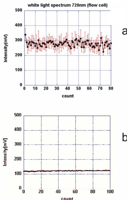
Figure 4-a and -b: White light stability before and after the improvements.
