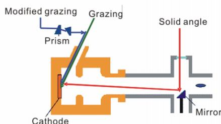
Figure 2: Laser injection techniques.
