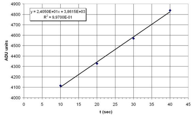
Figure 4: Grey level in ADU units versus exposure time showing the linearity of the imaging system.
