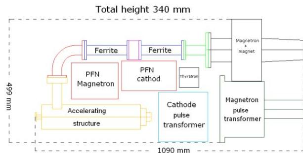
Figure 1: Design of a compact 5 MeV, S-band, 1 kW, electron linac for *in situ* applications.
