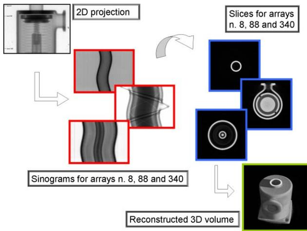
Figure 6: A schematic representation of the 3D image reconstruction procedure.
