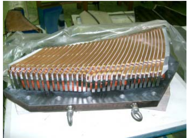
Figure 3: 32 trim coils attached to the pole piece of the injector.
