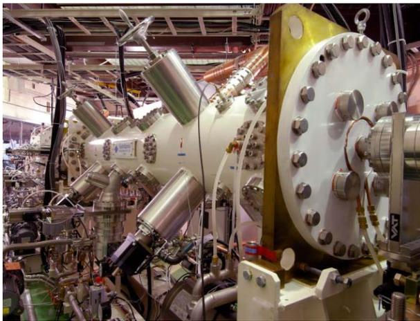
Fig. 2 A picture of the compact RFQ linac (a view from upstream).
