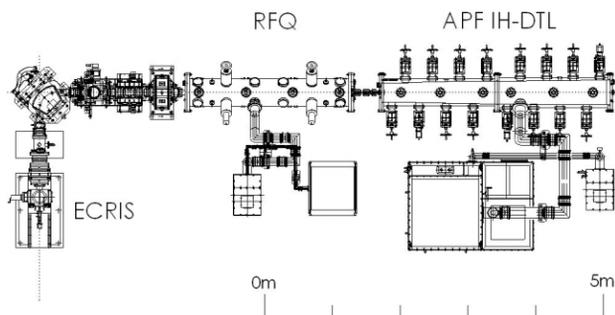
Figure 1: A schematic drawing of the compact injector.
