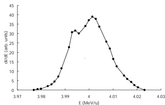
Fig. 5 A measured energy distribution of  $^{12}\text{C}^{4+}$ .
