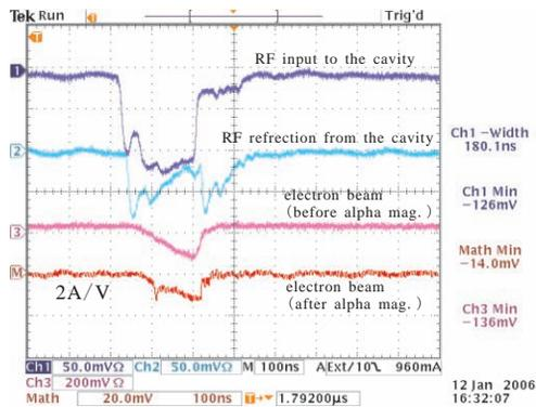
Figure 5: RF waveform propagating forward and reflected (upper two lines) from the gun cavity. The bottom two lines show the beam currents observed at the entrance and the exit of the alpha magnet, by a current transformer.
