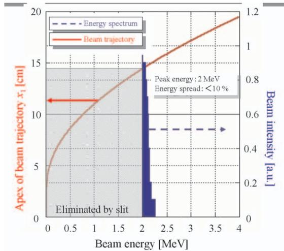
Figure 4: Energy spectrum of the electron beam measured by the alpha magnet (right-hand axis). The left-hand axis shows the apex of the beam trajectory in the alpha magnet.
