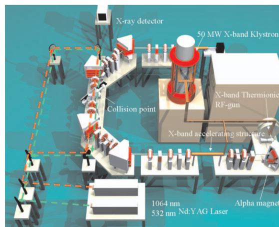
Figure 1: Schematic illustration of Compact Hard X-ray source based on thermionic-cathode X-band RF-gun, X-band accelerating structure and Q-switch Nd:YAG laser.
