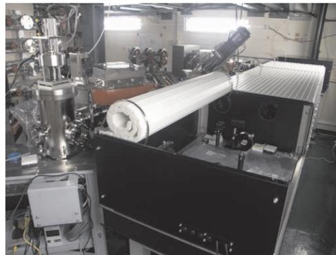
Figure 7: Photograph of the X-band linac beamline including the collision point and laser optics with laser pulse circulation system (LPCS).
