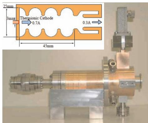
Figure 2: Photograph and schematic illustration(cut view) of the X-band RF-gun.
