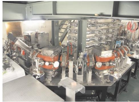
Figure 6: Photograph of the X-band linac beamline including the X-band RF-gun and alpha-magnet.
