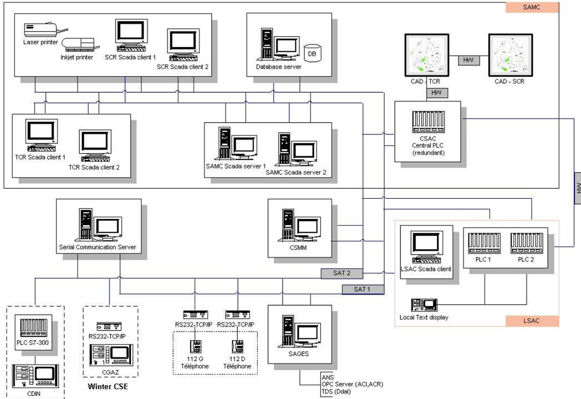
Figure 3: CSAM hardware architecture.
