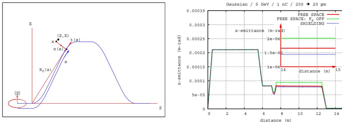
Figure 1: Left: lab frame  $(Z, X)$  and beam frame  $(s, x)$  for a chicane bunch compressor. Right: Normalized transverse emittance (x-emittance). In red free space case, in green free space case without transverse force, in blue with shielding. The values at the end of the chicane are 1.67 mm-mrad, 2.01 mm-mrad and 1.44 mm-mrad respectively.
