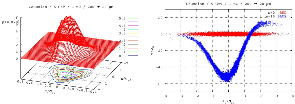
Figure 4: Left: perturbed charge density with shielding at  $s = 15m$  (end of chicane). Here  $\sigma_{z0} = 2mm$  and  $\sigma_{x0} = 0.64mm$ . Right: Scatter plots of the interaction picture variable  $w = p_{z0} - uz_0$  vs  $z_0$  at  $s = 15$ , where  $u$  is the slope in the initial  $p_z, z$  correlation. Here  $u = -36m^{-1}$  and  $\sigma_u = 2 \times 10^{-6}$ .
