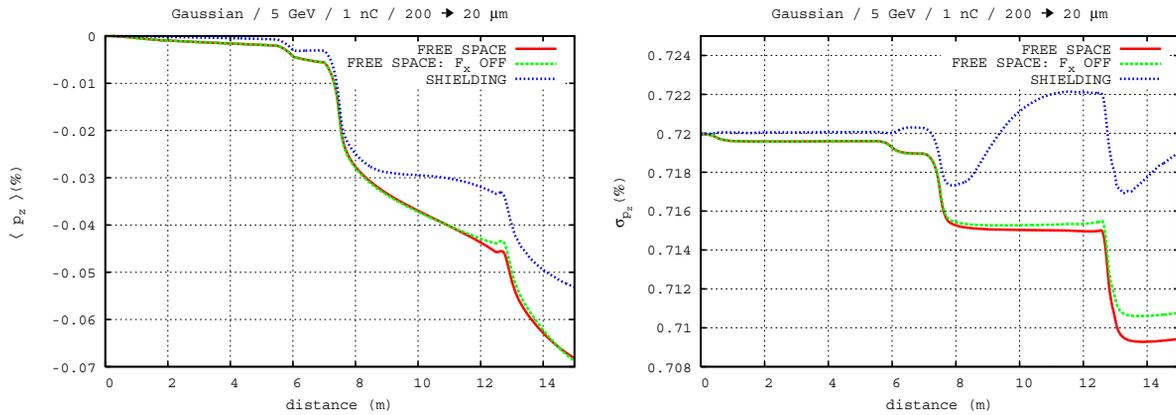
Figure 3: Left: mean of the relative energy loss. Right: standard deviation of the relative energy deviation. In red free space case, in green free space case without transverse force, in blue with shielding.
