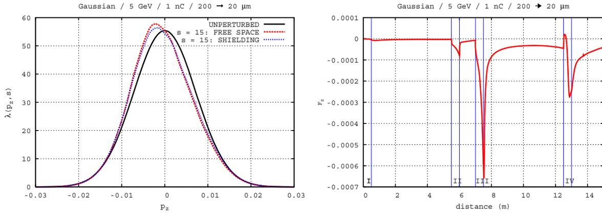
Figure 2: Left:  $\lambda(p_z, s)$ , the density in  $p_z$ . In black stationary unperturbed distribution, in green free space case at  $s = 15$  and in blue with shielding at  $s = 15$ . Right: mean of  $F_z$ . The magnets are indicated by I, II, III and IV.
