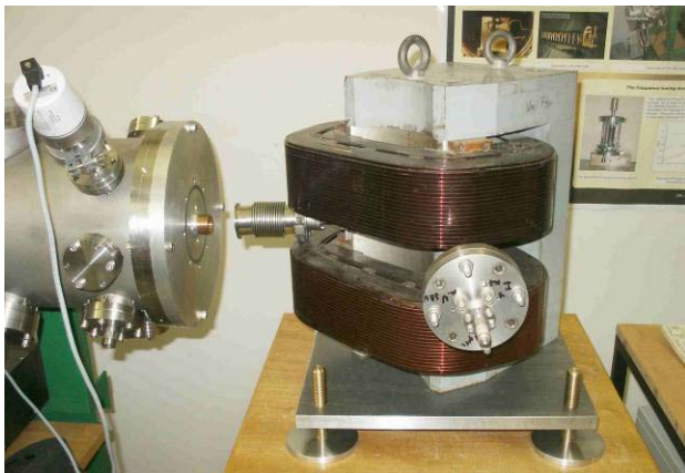
Figure 3: 90° bending magnet for impulse diagnostics.
