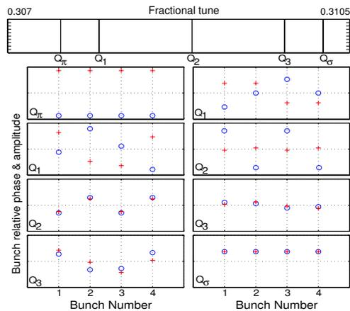
Figure 2: Eigenfrequencies and eigenvectors of a system of four bunches colliding head-on in two IPs.
