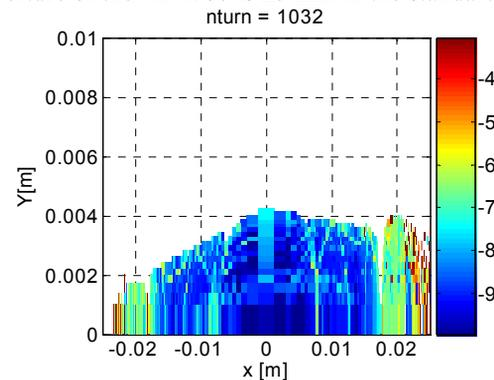
Figure 3: On-momentum DA with U23. The vertical aperture of the U23 is  $\pm 2.5$  mm in the standard straight.
