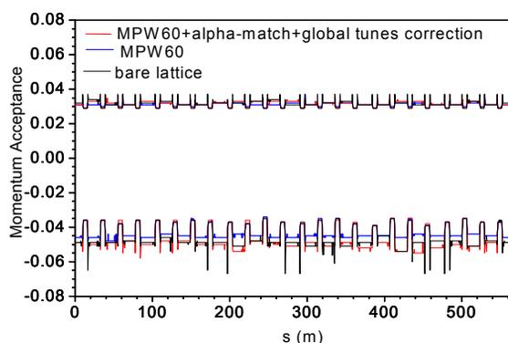
Figure 5: Comparison of 6D Momentum acceptance for the MPW60 with and without linear optic correction.
