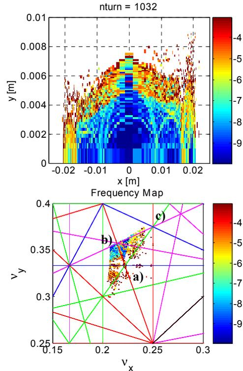
Figure 2: On-momentum DA and FM with MPW60 with alpha-matching/global tunes correction. The vertical aperture of the MPW60 is  $\pm 5$  mm in the standard straight.
