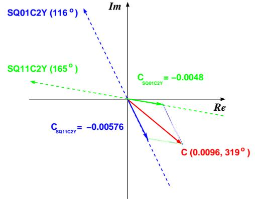
Figure 5: Sketch of the measured  $C$  decomposed on the axis defined by the two skew quadrupoles used for correction.
