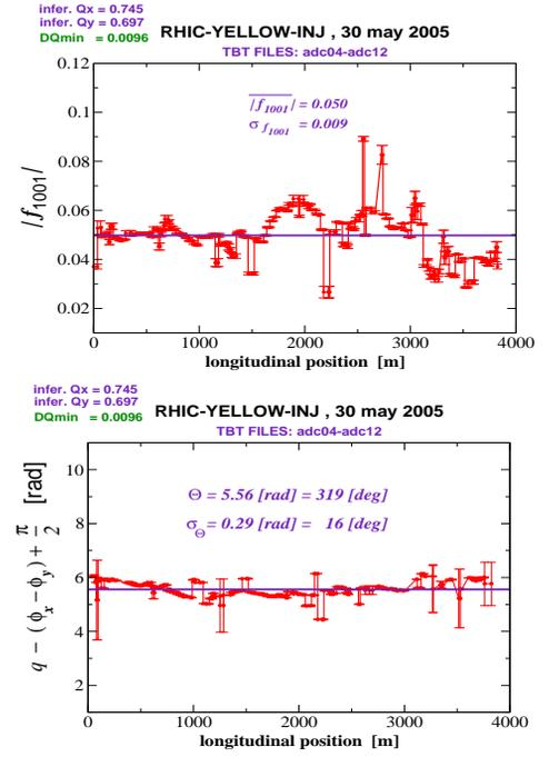
Figure 4: Variation along the Yellow ring at injection of  $|f_{1001}|$  (top) and  $q^w - (\phi_x^w - \phi_y^w) - \text{sgn}(\Delta) \frac{\pi}{2}$  (bottom). The corrector skew. Data points (i.e. BPMs) with fluctuation larger than 30% were rejected.
