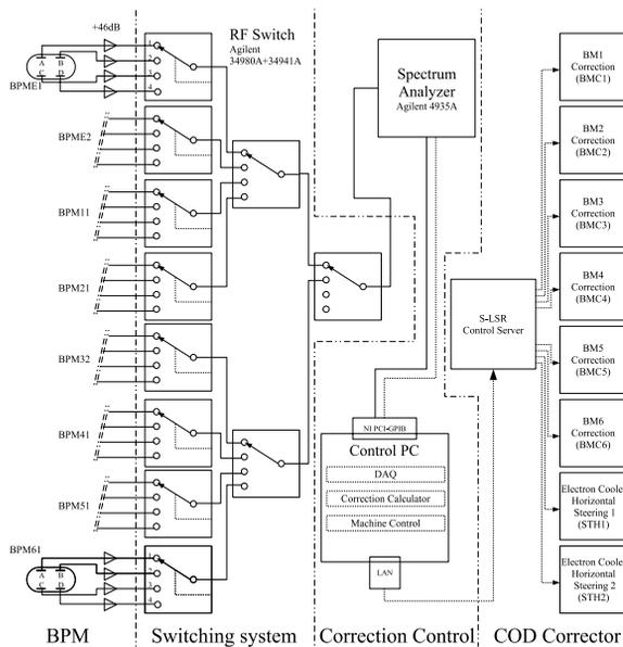
Figure 2: Block diagram of the COD correction system
