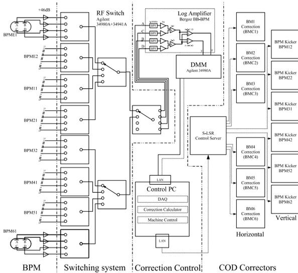
Figure 5: Block diagram of  $Mg^+$  COD correction
