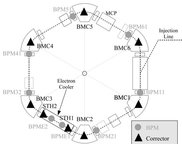
Figure 3: The layout of BPMs and correctors. BPMs are indicated as circles and correctors are triangles.
