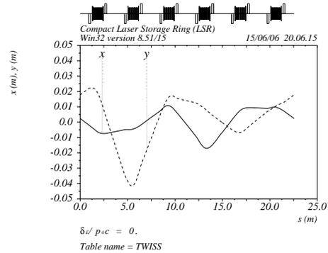
Figure 1: Calculated COD with electrode errors
