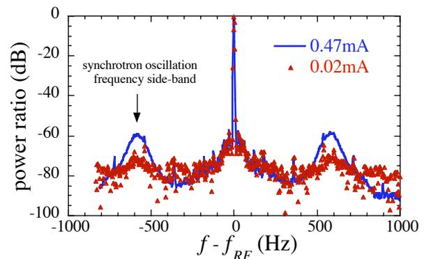
Figure 4: Beam current dependence of the synchrotron oscillation side-band. The main peak (rf frequency  $f_{RF}$ ) is normalized to 0dB. White noise was subtracted from the data at 0.02mA.
