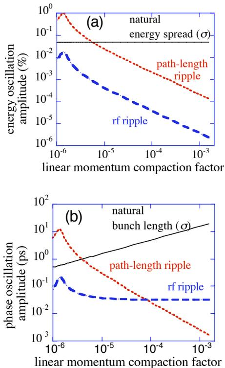
Figure 3: Estimation of (a) energy oscillation and (b) phase oscillation amplitude as a function of momentum compaction factor.
