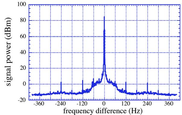
Figure 2: FFT power spectrum of the beam signal picked up from the button electrode. The center frequency is the rf frequency (500MHz).
