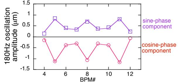
Figure 1: Horizontal oscillation amplitudes of 180Hz components at 9 BPMs. The lines are fitted function assuming 180Hz deflections at the magnets by the two power supplies, one for invert bends at the eastern arc and another for those at the western arc.
