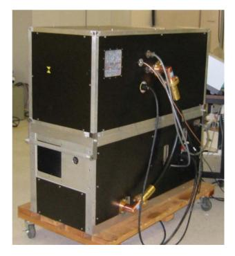
Figure 3: Portable Model PL-2 linac neutron generator.
