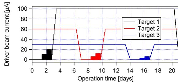
Figure 2: Driver beam current over a three-week period for different nominal intensities at each of the three target stations.
