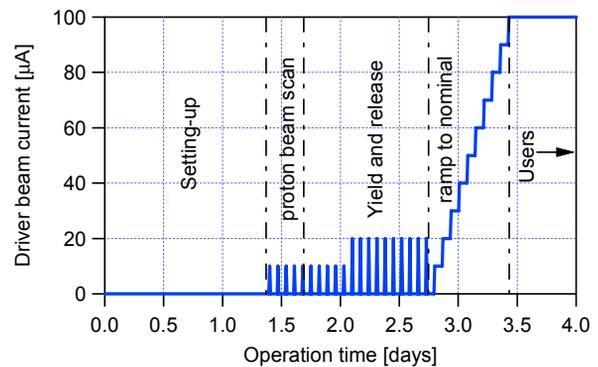
Figure 1: Target operation stages including setting-up, proton beam scan, yield and release measurements, ramping up to nominal current and handing over to users.
