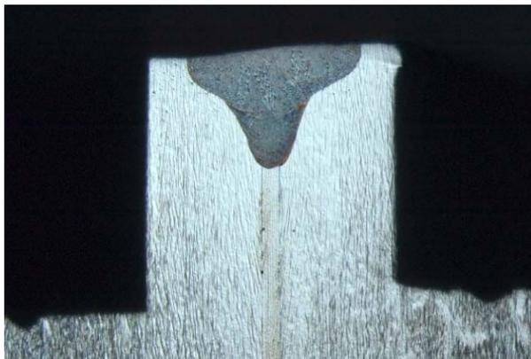
Figure 1: Micrograph showing the EB weld geometry
