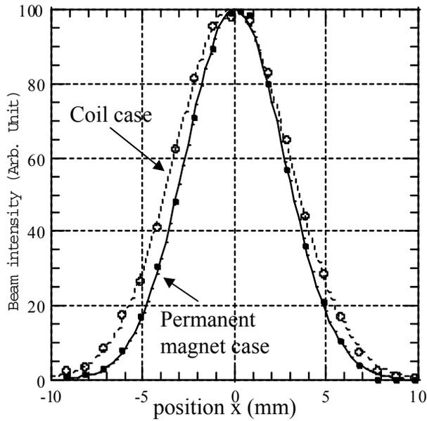
Figure 5: Spatial distribution of the extracted ion beam
