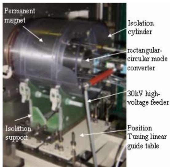
Figure 3: Photograph of the permanent magnet microwave ion source
