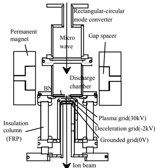
Figure 2: Schematic of the permanent magnet microwave ion source
