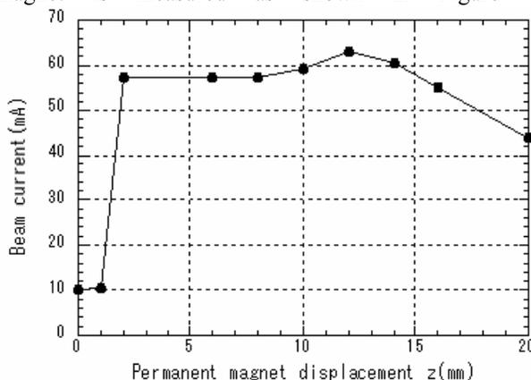
Figure 4: Dependence of beam current on displacement of permanent magnet
