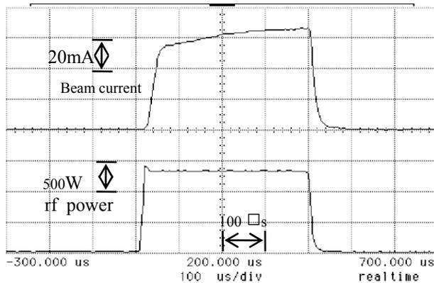
Figure 6: Pulse waveforms of beam current and rf power
