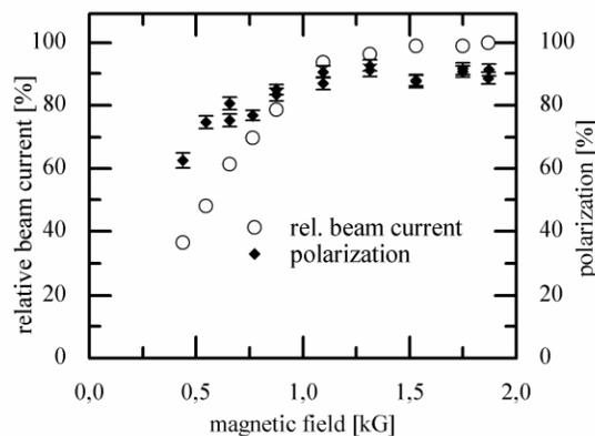
Figure 3: Beam intensity as a function of the magnetic field magnitude in the charge exchange solenoid.
