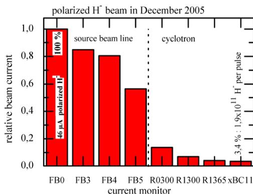
Figure 6: Record beam transport from the polarized ion source and ions per pulse for injection into COSY.
