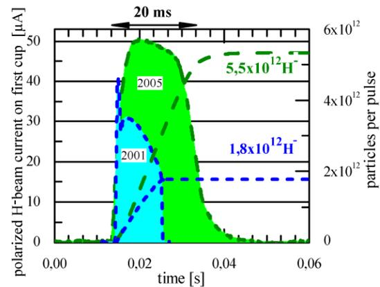
Figure 5: Record beam pulses from the polarized ion source and integrated particle number per pulse.
