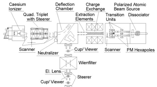
Figure 1: Layout of the COSY CBS. Being underlined indicates added or replaced parts.
