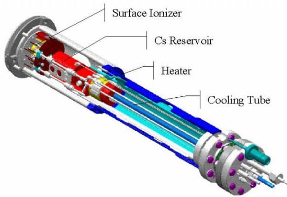
Figure 2: Pulsed Caesium ionizer. Only the main parts are shown.
