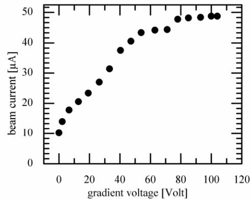
Figure 4: Beam intensity as a function of the magnitude of the gradient voltage applied over the charge exchange region.
