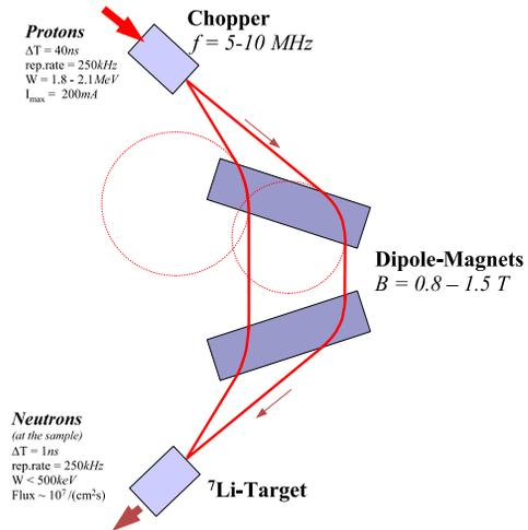
Figure 2: *1ns*-Buncher-System. A bending system composed of two skew magnets with spatial non-constant magnet fields would have several advantages, e.g. more parameters in order to manipulate the beam dynamics, in average a greater distance between two bunches and a more compact geometry.
