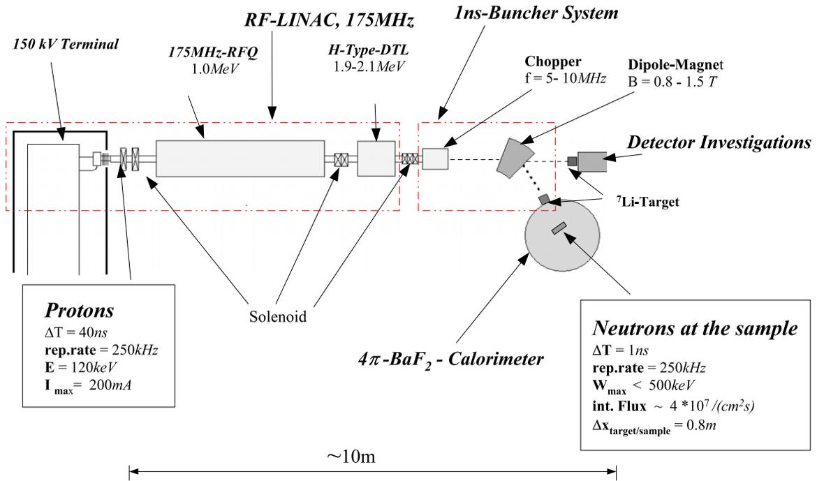
Figure 1: Sketch of FRANZ.  $\Delta T$  is the length of one macro bunch. The distance between the  ${}^7\text{Li}$ -target and the sample is given by 0.8m. The single bending magnet in this figure is just a symbol for a more complicated bending system. (see Fig.2)
