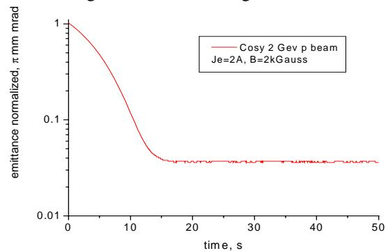
Figure 1: Normalized beam emittance versus time at electron cooling of 2 GeV proton beam (without target, parameters see text).
