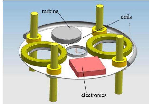
Figure 3: Layout of a complete high voltage section.
