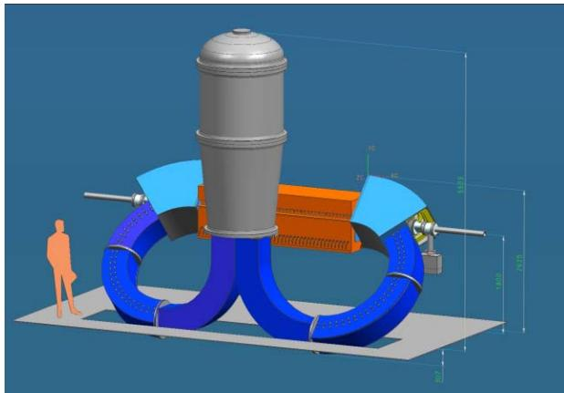
Figure 2: Layout of the proposed 2 MeV electron cooler for COSY.
